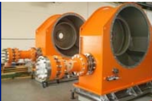
2 single-nozzle Pelton turbines during works assembly
