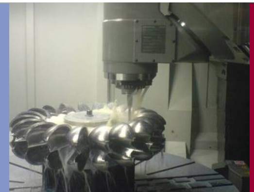
Milling of Pelton runner
