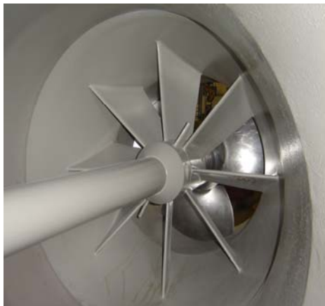
The special hydraulic design of wicket gate and runner is responsible for the self cleaning mechanism
